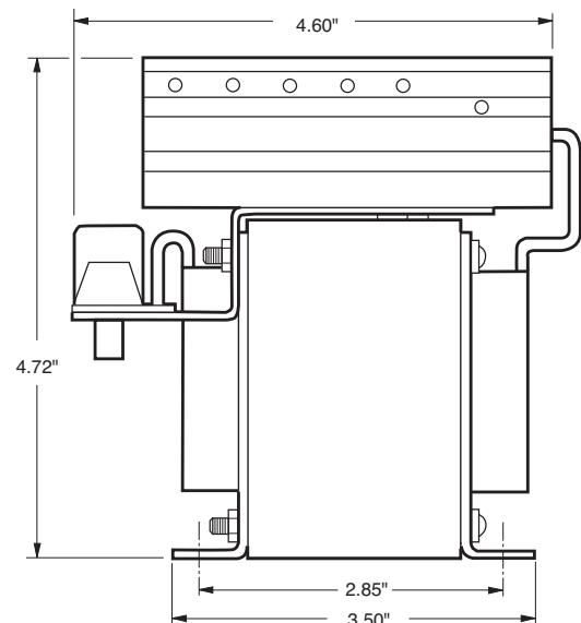
This control may be mounted on its base (two mounting slots) or on its back (four mounting slots).
